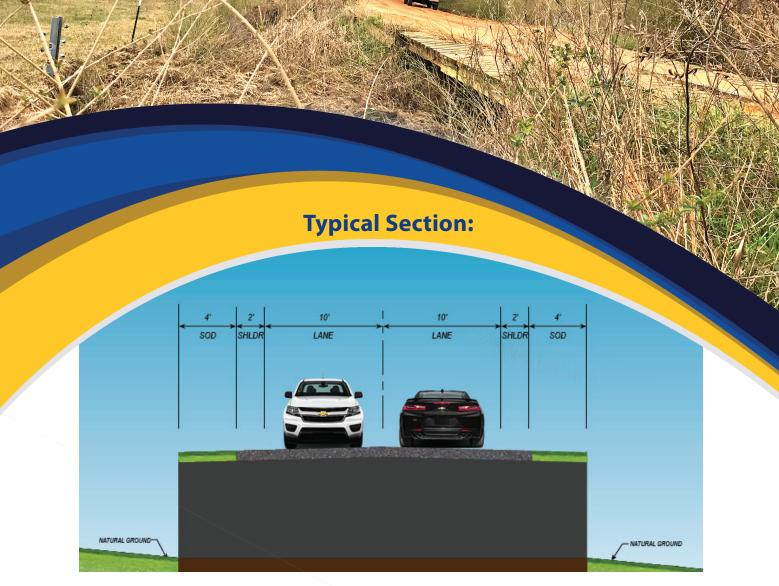
The two-lane concrete box culvert will provide a ten-foot wide travel lane with a two-foot wide shoulder in each direction.
