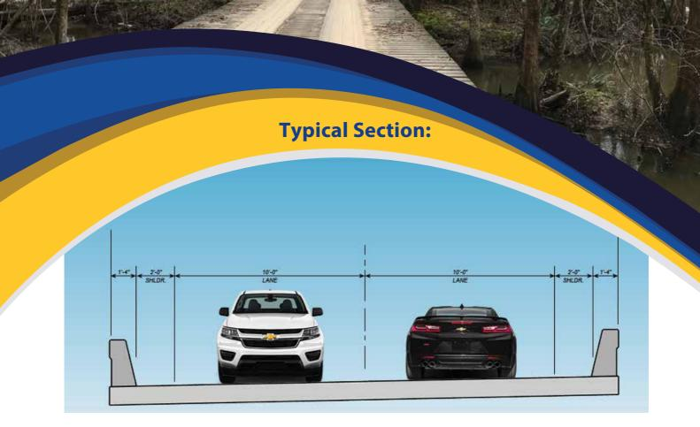
The two-lane concrete bridge will provide a ten-foot wide travel lane with a two-foot wide shoulder in each direction.
